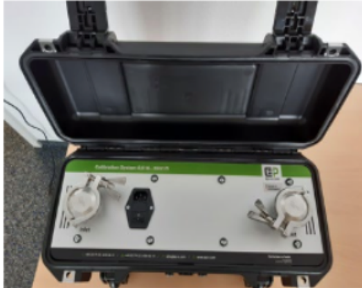
① Mobile measuring box with integrated gas meter for use on site
